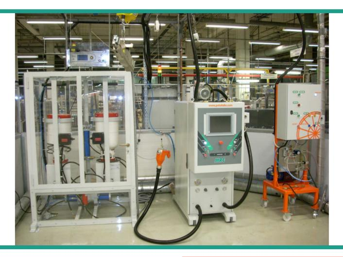
The VTech MRC-HC Automatic Evacuation and Refrigerant Charging System is designed for safely and accurately charging HC refrigerants (e.g. R290, R600a, R170 or R32) in a production environment. The system also performs an automatic vacuum cycle and a vacuum decay leak test, prior to refrigerant charging.
